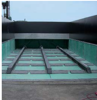
Plastic lining, stainless steel push frame series ZBC
