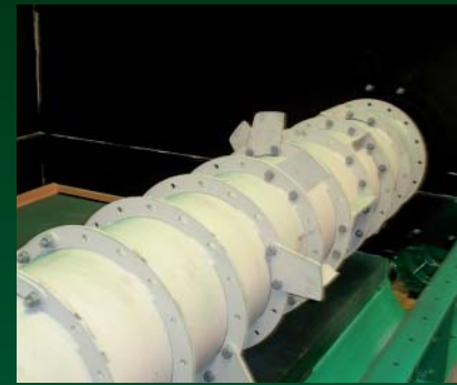
Dosing and disintegrating roller with replaceable tools made of stainless steel
