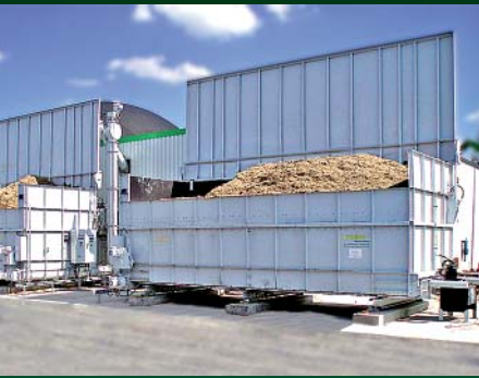
Solid matter dosing systems with hydraulically operated cover series SBC, 80 m 3
