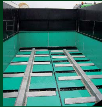
Plastic lining, stainless steel push floor series SBC
